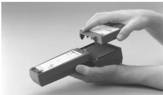
FIGURE 1-43. Battery Pack Removal.
