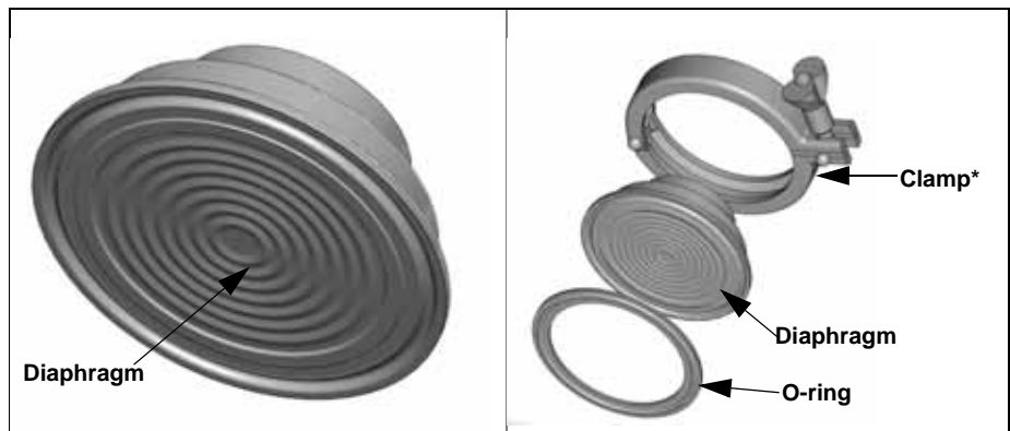
Figure 3-27. Hygienic Tri-Clamp Remote Seal 3-D Diagram
