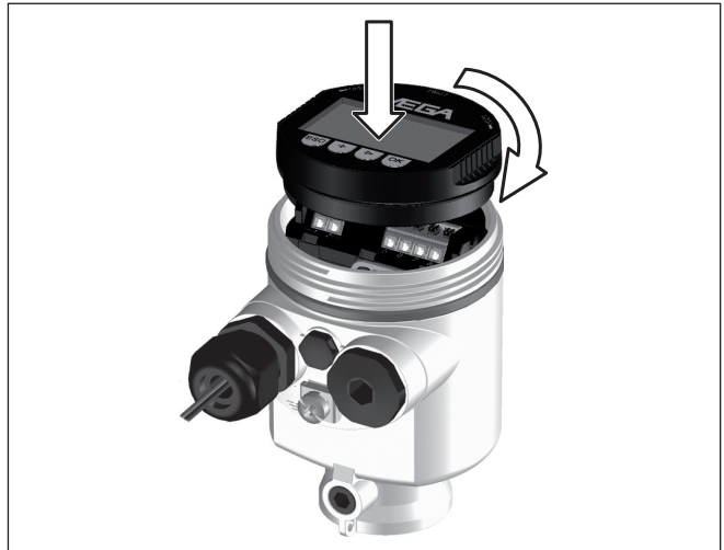
Fig. 22: Insertion of the indicating and adjustment module with single chamber housing into the electronics compartment
