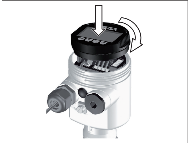
Fig. 24: Insert display and adjustment module
